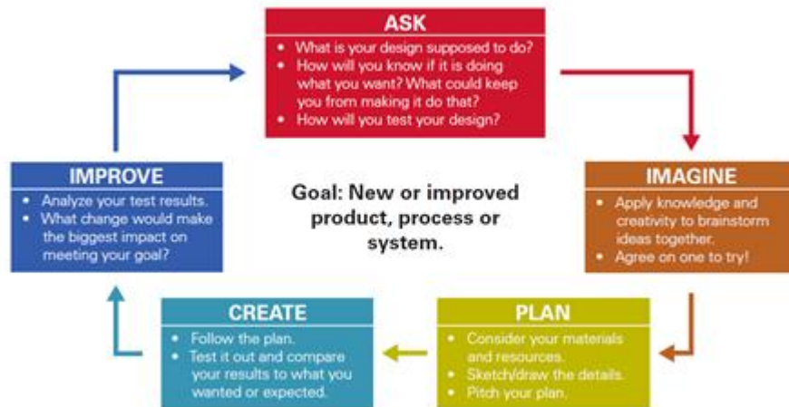
Figure 2. Five-Step Model of Engineering Design Process (NC State University, 2019)
